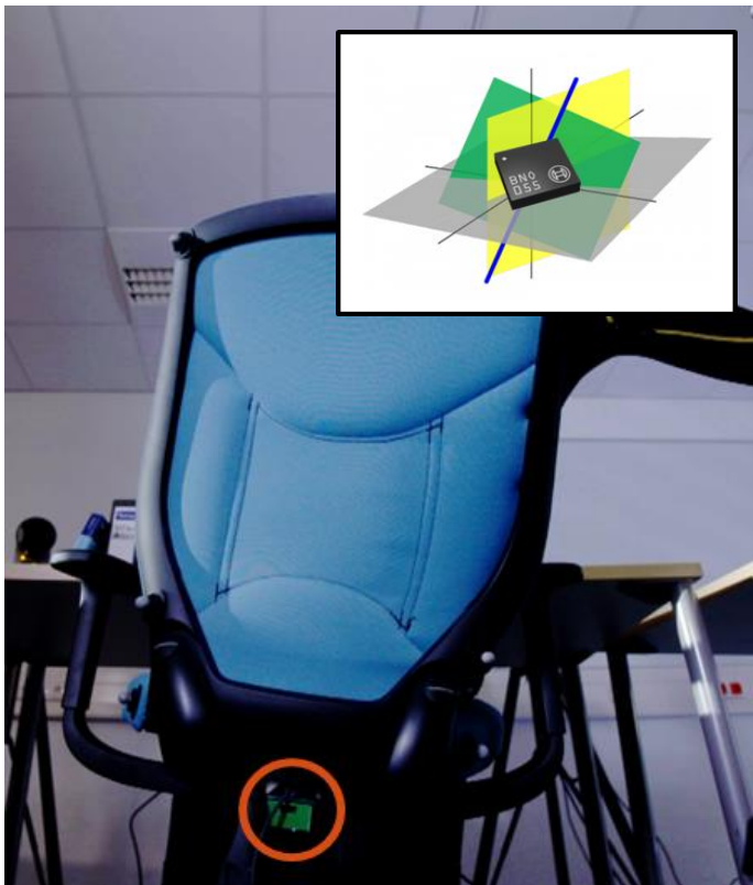
Figure 6: Position of the orientation sensor underneath the office chair and diagram of the measurement levels
