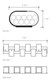
Wilkhahn cable claws are used to hold and direct cables horizontally underneath the work surface.
